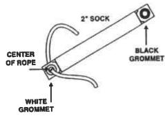
Wrap each end of the installation rope around the sock twice and then cross them through the black grommet.
