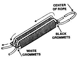
1. Find the center of the rope. Begin lacing the ORC Socks by threading the two ends of the installation rope through the black grommets and then through the white grommets at the bottom of the same side of the bottom sock
