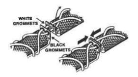
5. To avoid the ORC Sock slipping past each other, the socks must be laced with the grommet flaps of the bottom sock and second sock butting against each other (as shown)
