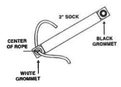
Find the center of the rope. Begin lacing the ORC Socks by threading one end of the installation rope through the white grommet, make sure that the center of the rope is pulled through to the center of the white grommet on the bottom sock.
