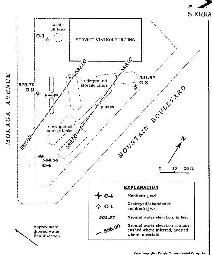
Figure 1. Monitoring Well Locations and Ground Water Elevation Contour Map - March 2, 1994 - Chevron Service Station #9-1740, 6550 Moraga Avenue, Oakland, California
