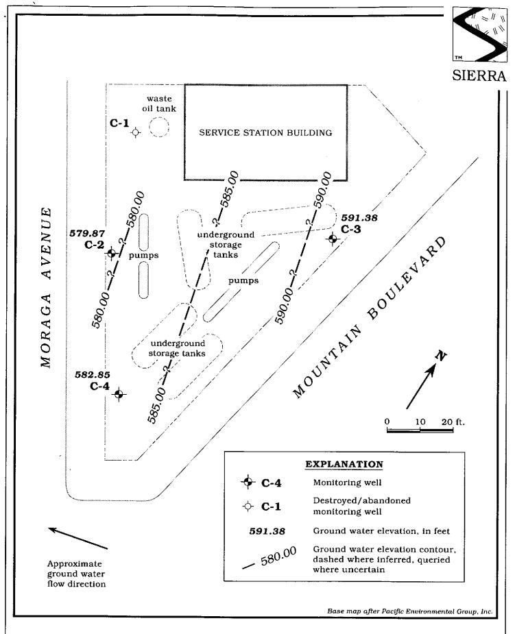
Figure 1. Monitoring Well Locations and Ground Water Elevation Contour Map - December 6, 1993 - Chevron Service Station #9-1740, 6550 Moraga Avenue, Oakland, California
