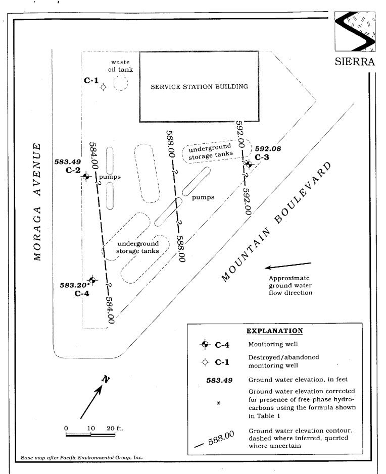
Figure 1. Monitoring Well Locations and Ground Water Elevation Contour Map - March 30, 1993 - Chevron Service Station #9-1740, 6550 Moraga Avenue, Oakland, California
