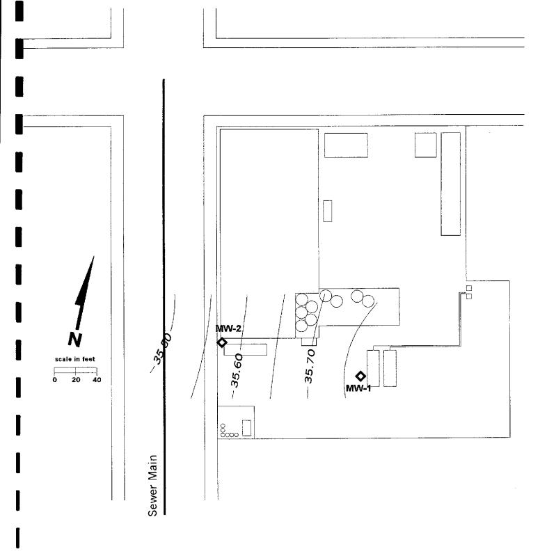
Figure 3: Groundwater Elevations Contour Map Based on April 6, 2000 Monitoring Data
