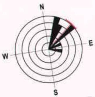
Shell Groundwater Gradient Direction
