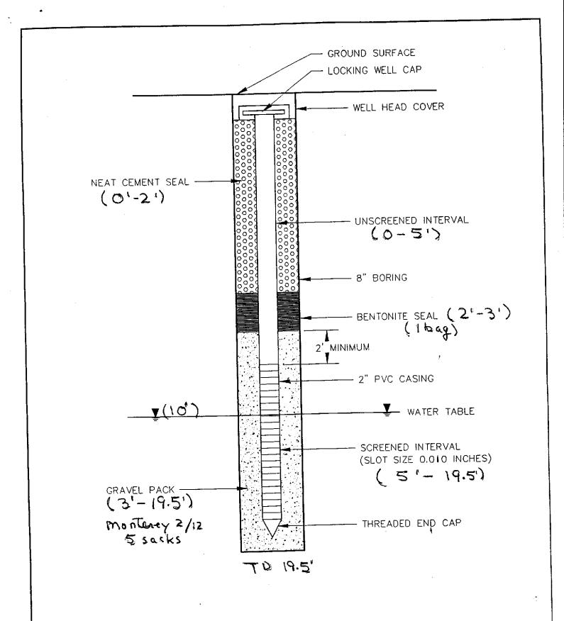
Well No: MW-1, Mission Valley Rock, 799 Athenour Way, Sunol; Construction Diagram 6-18-98
