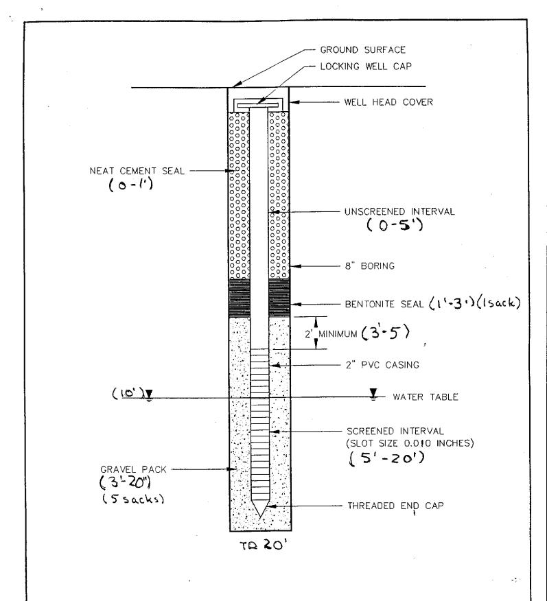
Well No: MW-2; Mission Valley Rock, 799 Athenour Way, Sunol; Construction Diagram 6-18-98
