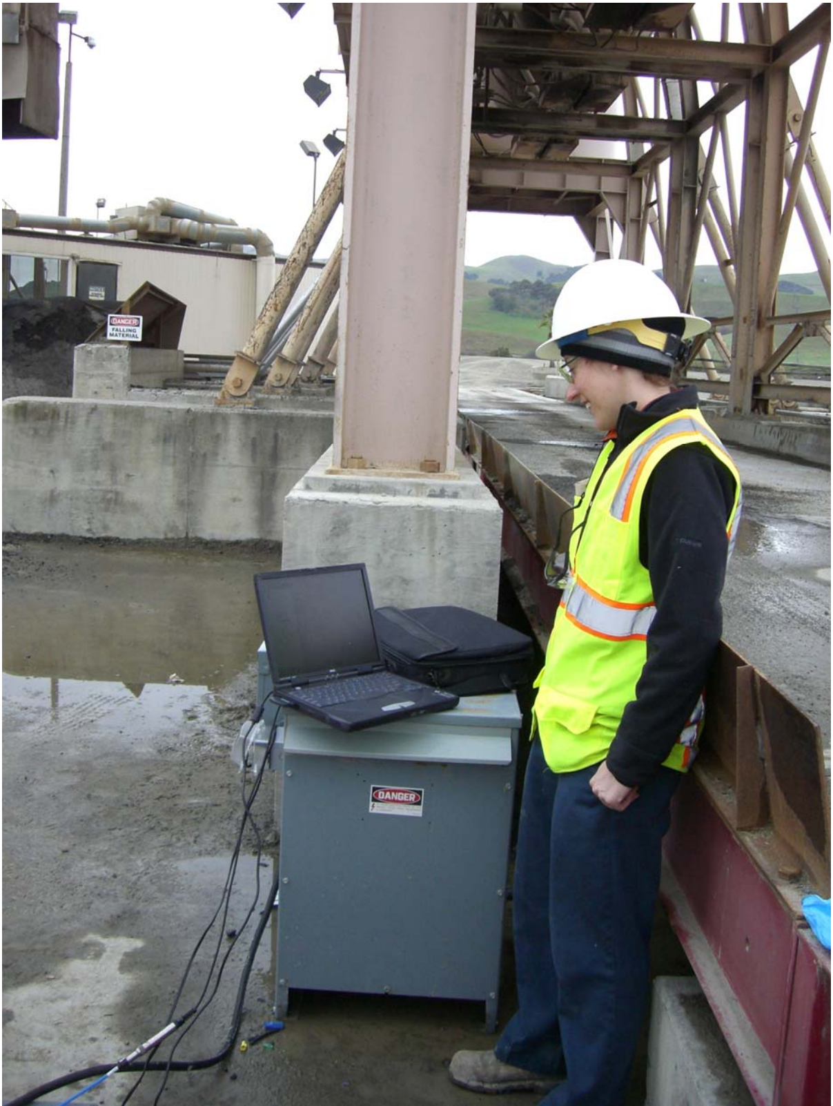
Photograph 3: Uploading Data from an In-Situ® 9500 TROLL to a Laptop Computer.
