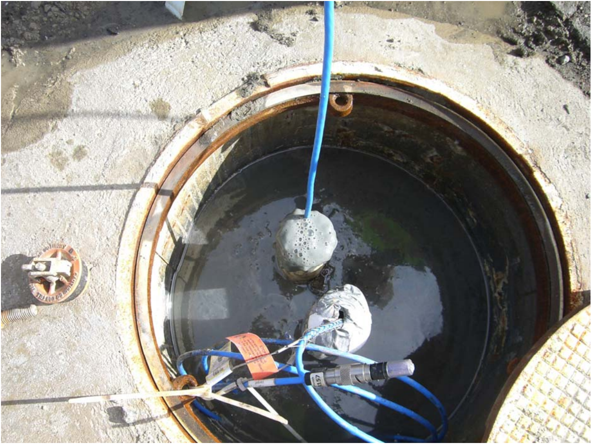
Photograph 5: Silt-Laden Water Bubbling Over From Monitoring Well MW-7D During Sparging of OXY-1D and OXY-1LF Simultaneously. Blue Cables are Attached to Down-Hole In-Situ® 9500 TROLLs.
