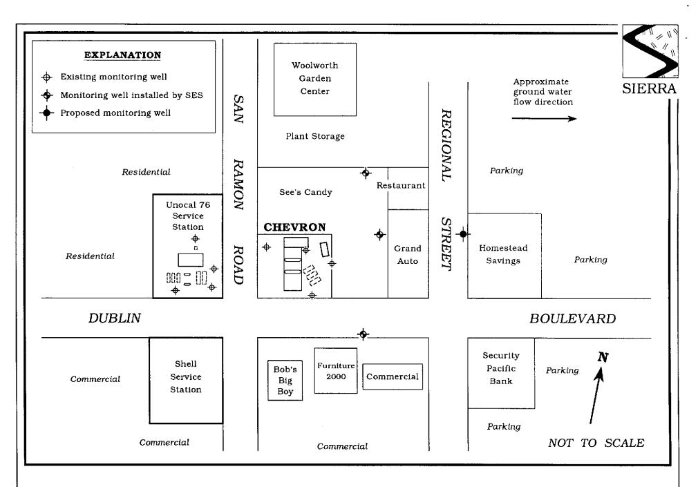
Figure 3. Proposed Monitoring Well Location Map - Chevron Service Station #9-5542, 7007 San Ramon Road, Dublin, California
