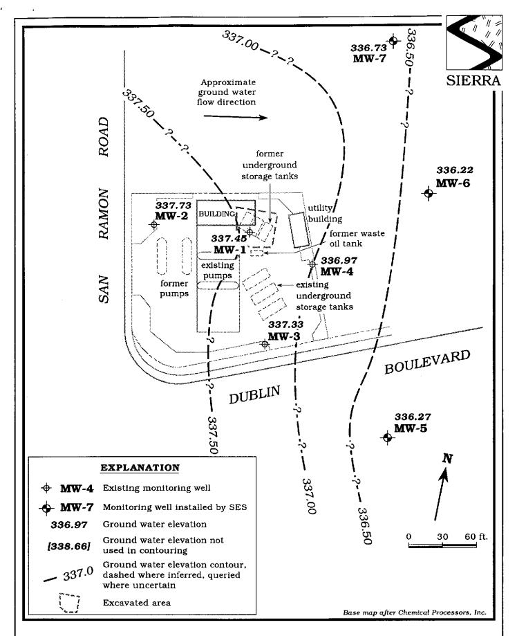
Figure 2. Monitoring Well Location and Ground Water Elevation Contour Map – July 17, 1991 – Chevron Service Station #9-5542 – 7007 San Ramon Road, Dublin, California
