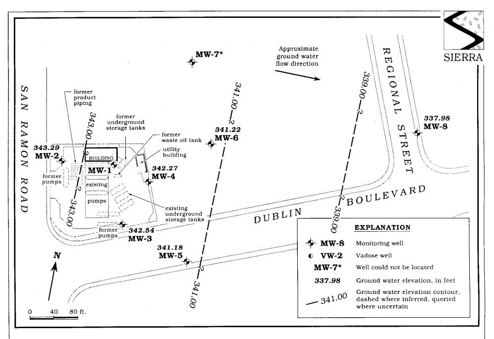
Figure 1. Monitoring Well Location and Ground Water Elevation Contour Map - March 22, 1993 - Chevron Service Station #9-5542, 7007 San Ramon Road, Dublin, California
