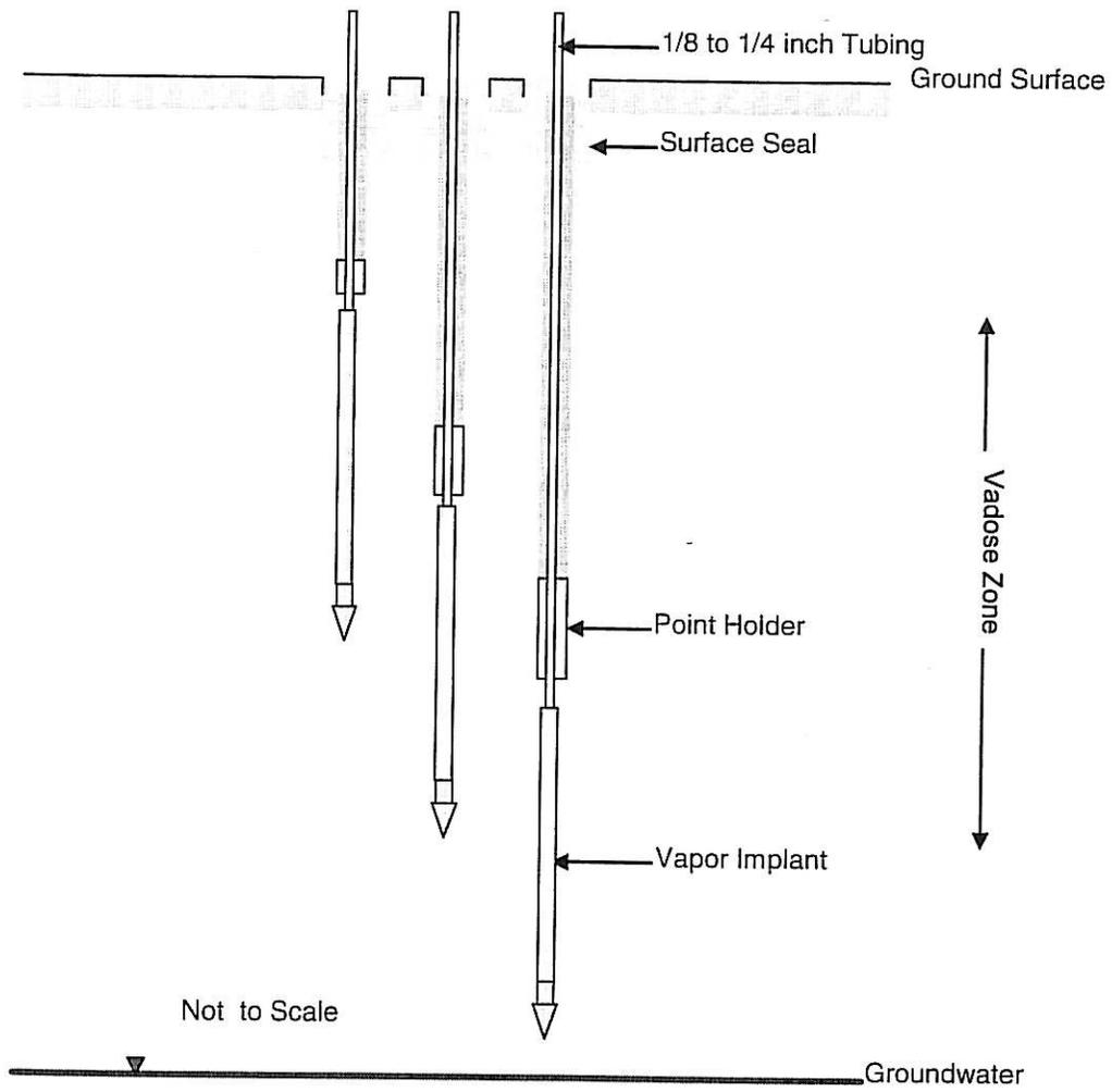
**Figure C-6.** Direct push permanent soil gas probe installation (developed based on illustration provided at [www.geoprobe.com](http://www.geoprobe.com)).
