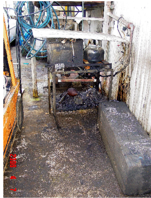
PHOTO 4. Oily metal shavings: Metal shavings, some apparently mixed with waste oil, were observed scattered on the Site's floor.
