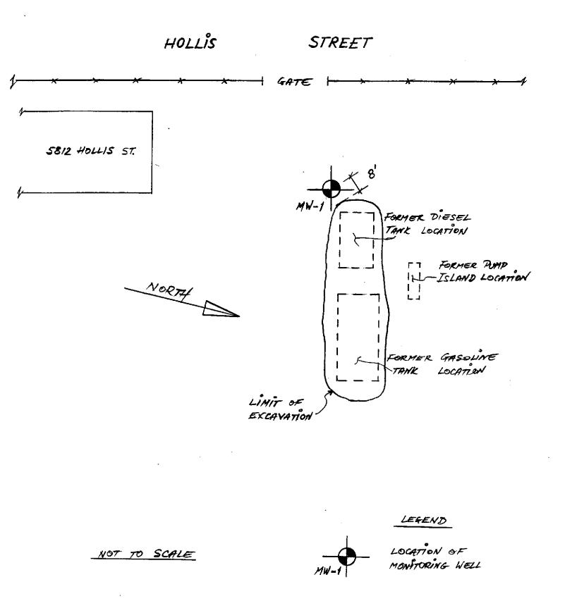
FIGURE 2 - SITE PLAN AND WELL LOCATION
