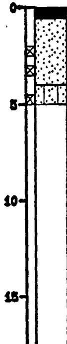
3" ASPHALT, 3" GRAVEL SUBBASE
