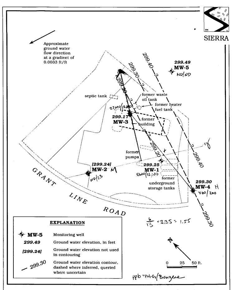
Figure 2. Monitoring Well Locations and Ground Water Elevation Contour Map - 1944 - Former Chevron Service Station #9-7127, Interstate 580 and Grant Line Road, Altamont Pass, California
