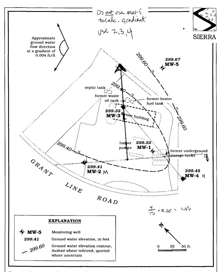
Figure 1. Monitoring Well Locations and Ground Water Elevation Contour Map - 1994 - Former Chevron Service Station #9-7127, Interstate 580 and Grant Line Road, Altamont Pass, California
