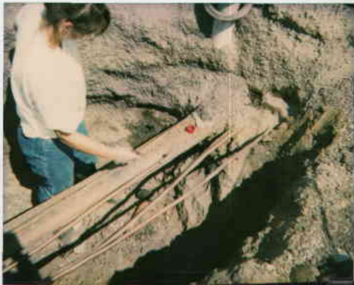
7/19/93-Photo taken by Ron Oweasz at Banzal Shell, 2120 Montana Ave, Oak. Shown is Allison Watts taking soil samples after pit reexcavation. ©
