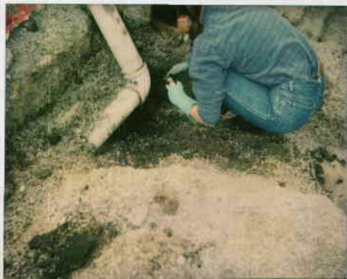
7/6/93-Photo taken by Ron O'Carroll at Bansal shell, 2120 Montana Ave, Oak. Shown is Allison Watts taking soil sample at end of old piping where some soil cont. was observed. @
