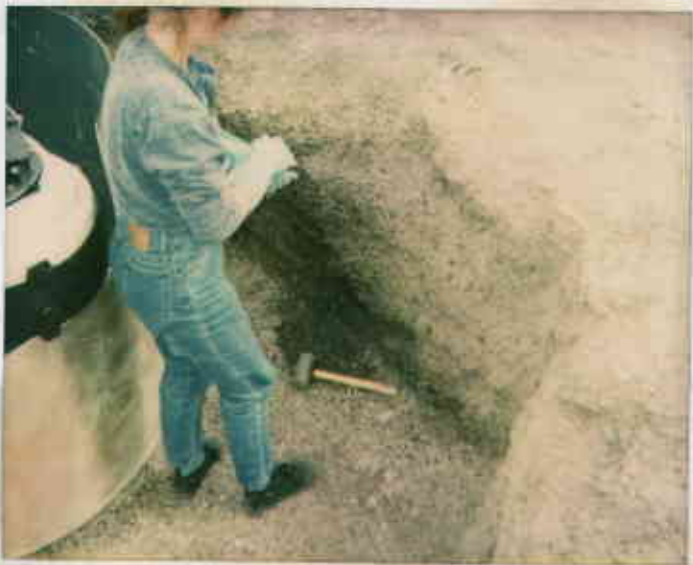
7/6/93-Photo taken by Ron O'Carroll at Bansal shell, 2120 Montana Ave, Oak. Shown is Allison Watts taking soil sample in side wall of pit where cont. was found at UGT piping mod. @
