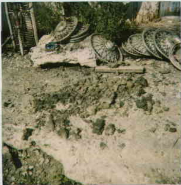
3744 Depot Rd, Hayward 8/29/95 Soil Cuttings from this boring at gas pit. Soil had strong petrol odor
