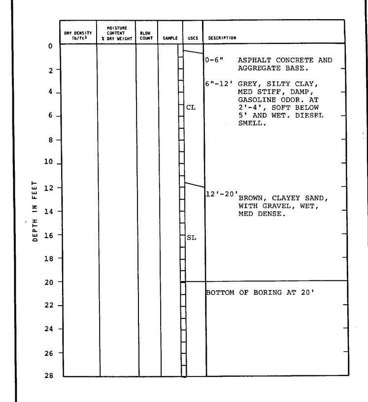
**PLATE** IT ENVIROSCIENCE/CHEVRON J.H. KLEINFELDER & ASSOCIATES OAKLAND, CALIFORNIA GEOTECHNICAL CONSULTANTS . MATERIALS TESTING 5 LOG OF BORING NO. B-2 PREPARED BY: PLC DATE: 3 /82 B-1189-1 PROJECT NO. DATE: 3/82 CHECKED BY: DCM
