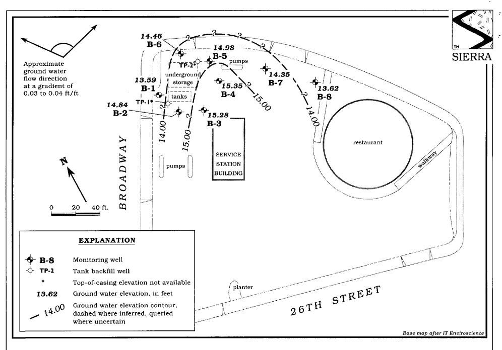
Figure 1. Monitoring Well Locations and Ground Water Elevation Contour Map - March 17, 1994 - Chevron Service Station #9-2506, 2630 Broadway, Oakland, California
