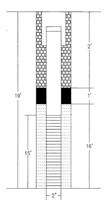
Schematic Diagram for Monitoring Well MW-23 SOUTH SHORE SHOPPING CENTER Corner of South Shore Drive and Park Street Alameda, Cal fornia
