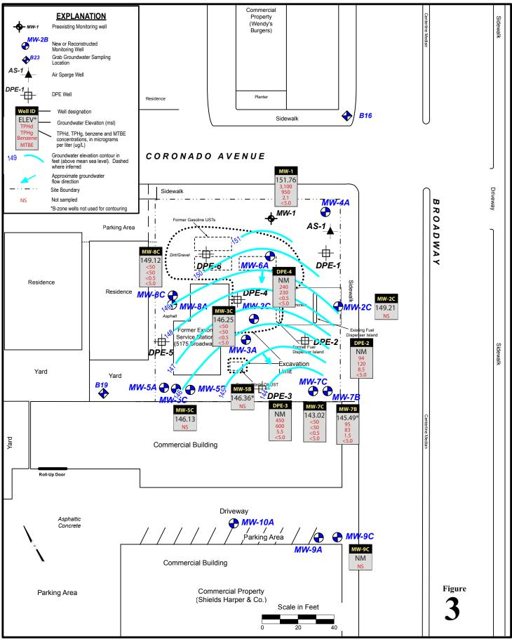
Former Exxon Station 5175 Broadway Oakland, California Groundwater Elevation Contour and Hydrocarbon Concentration Map (Deep) December 29-30, 2011
