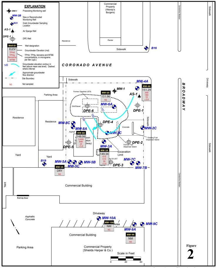
Former Exxon Station 5175 Broadway Oakland, California Groundwater Elevation Contour and Hydrocarbon Concentration Map (Shallow)
