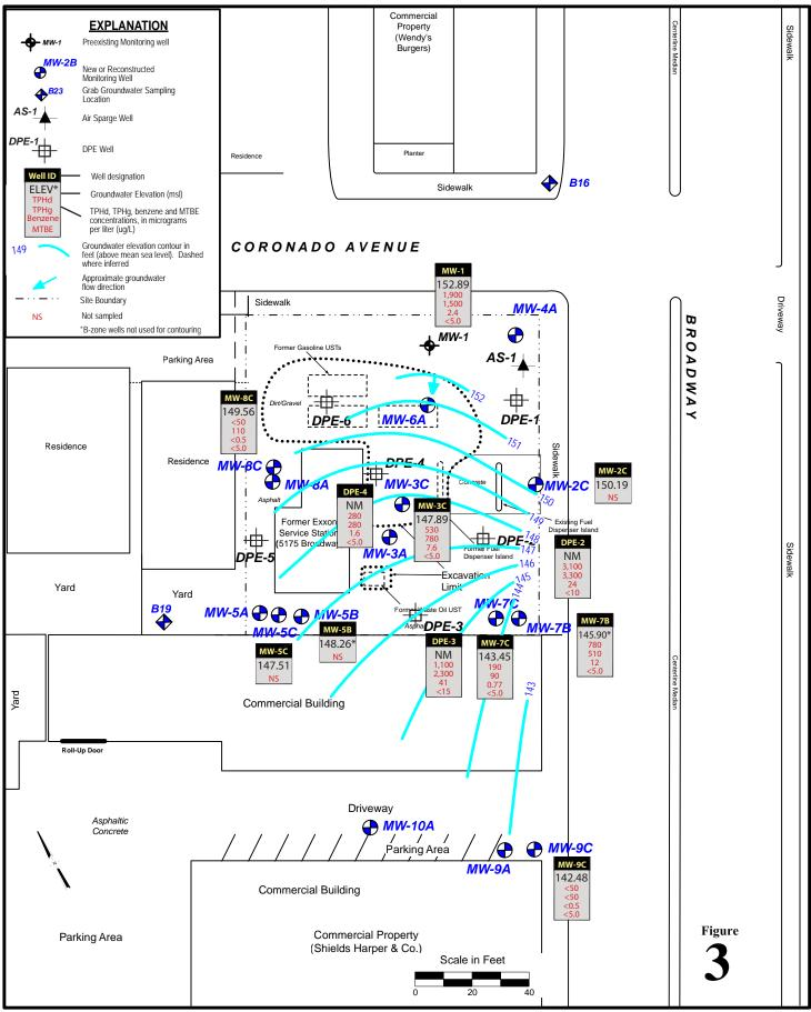
Former Exxon Station 5175 Broadway Oakland, California Groundwater Elevation Contour and Hydrocarbon Concentration Map (Deep) June 10, 2011
