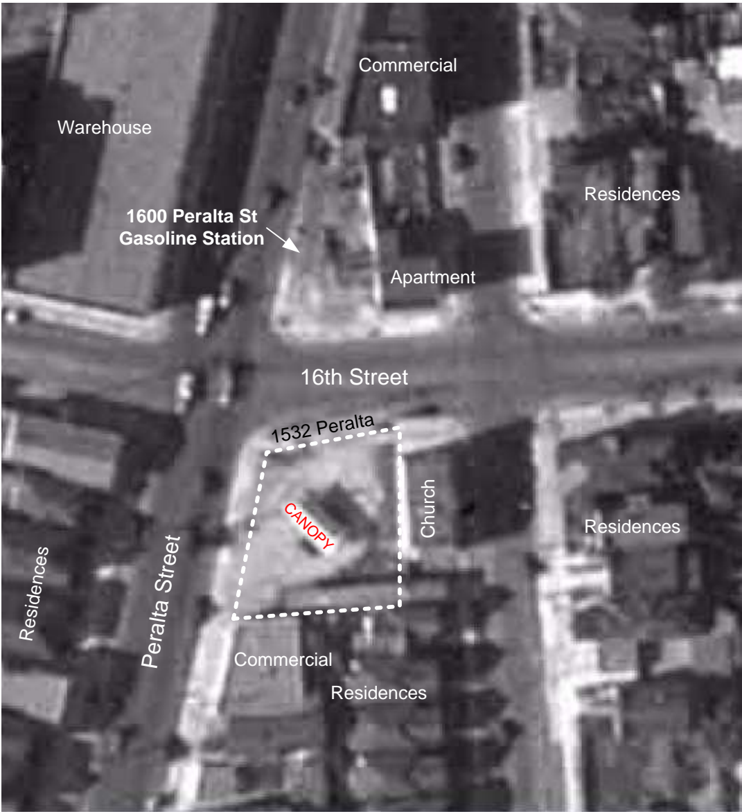
Enlarged portion of 1931 aerial photograph at an original scale of 1"=266 feet (Fairchild). North is to top of photograph. Subject property at 1532 Peralta St. is shown by dashed outline. Fueling station canopy present over location of dispenser island with office, rest room and oil storage building present along south margin of Site. Former gasoline station at 1600 Peralta St. is present in this 1931 aerial photo. Much of the surrounding neighborhood is similar to existing conditions. Aerial photo from The EDR Aerial Photo Decade Package dated January 9, 2007.
