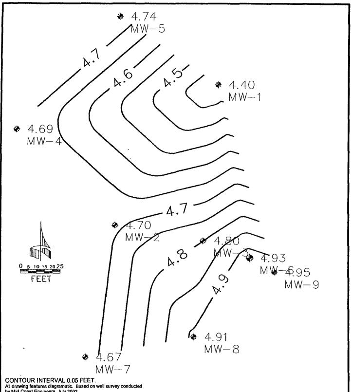
All drawing features diagramatic. Based on well survey conducted by Mid Coast Engineers, July 2002.
