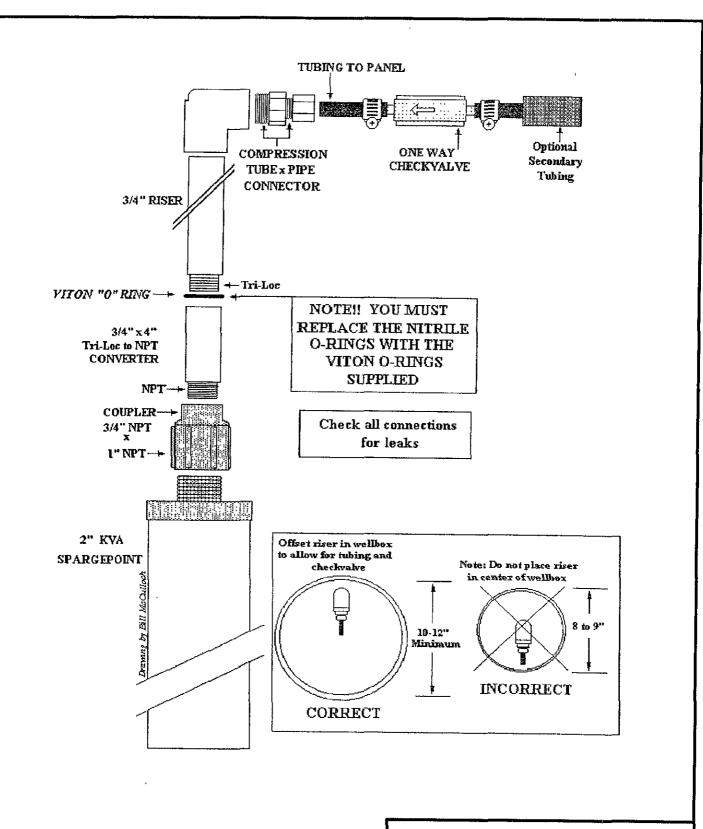
MANIFOLD TO WELL PLUMBING CONNECTION
