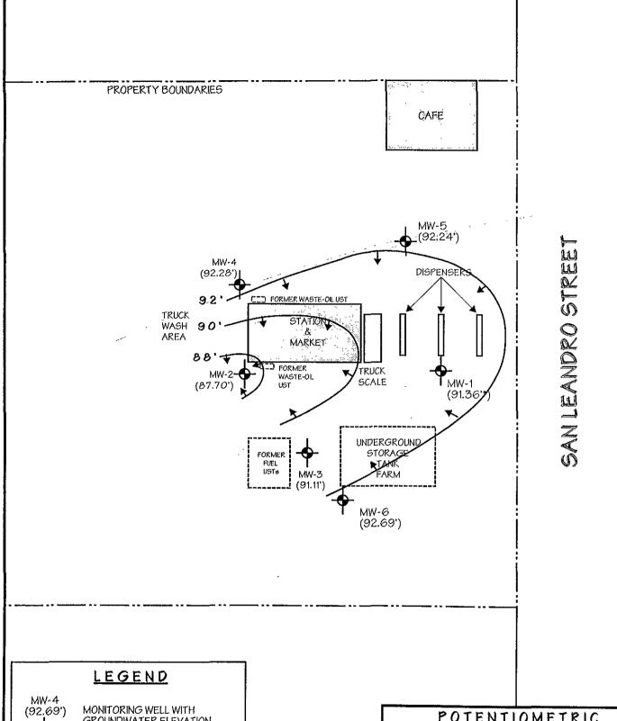
**GROUNDWATER ELEVATION** IN FEET, ABOVE MEAN SEA LEVEL
