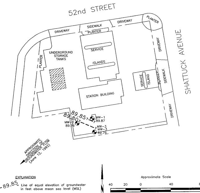
89.87 = Elevation of groundwater in feet above MSL June 12, 1992
