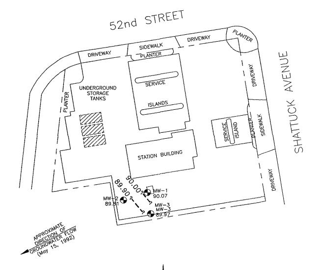
90.00 = Line of equal elevation of groundwater in feet above mean sea level (MSL)
