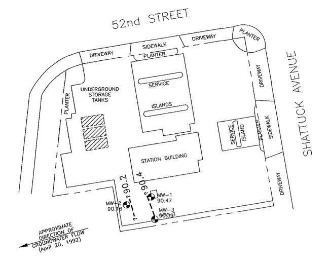
90. A = Line of equal elevation of groundwater in feet above mean sea level (MSL)
