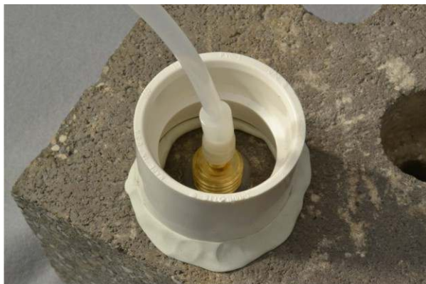
Figure 6. Water dam used for leak detection.
