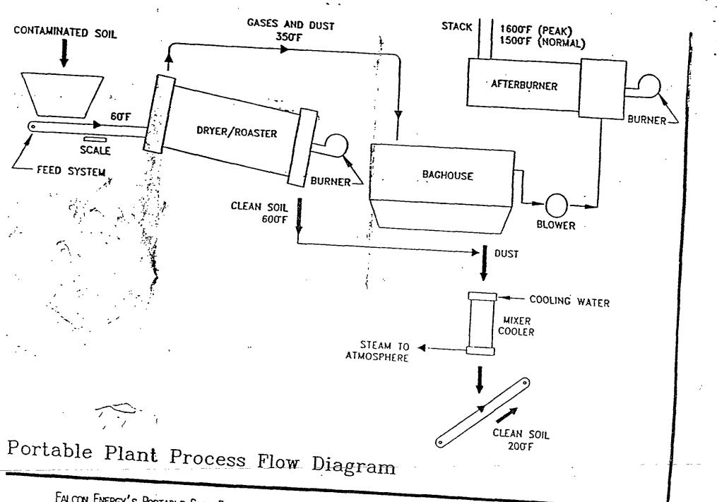
FALCON ENERGY'S PORTABLE SOIL REMEDIATION UNIT FOR HYDROCARBON CONTAMINATED SOILS
