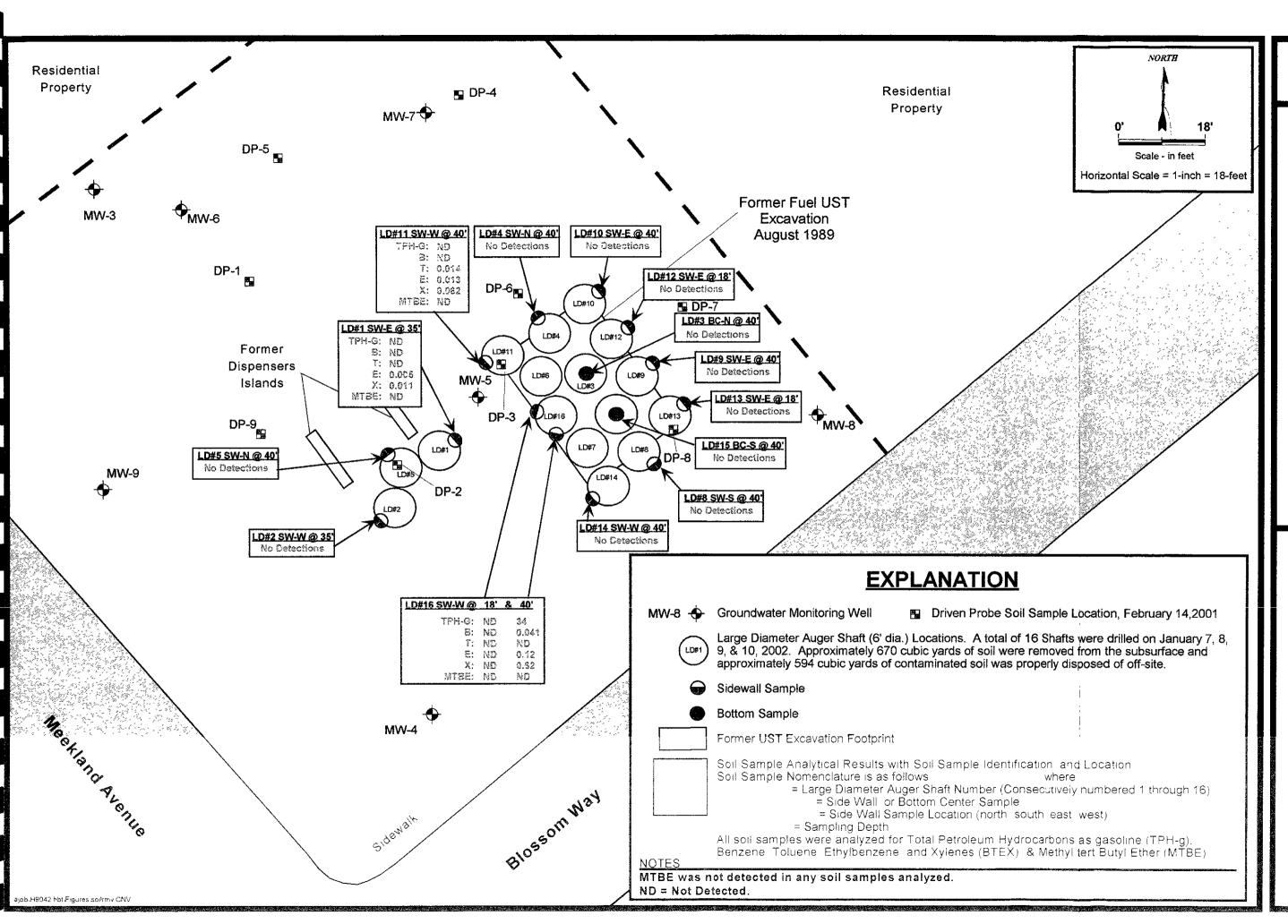
Large Diameter Auger Source Removal Footprint Map and Soil Sample Analytical Results Harbert Transportation 19984 Meekland Avenue Hayward, California
