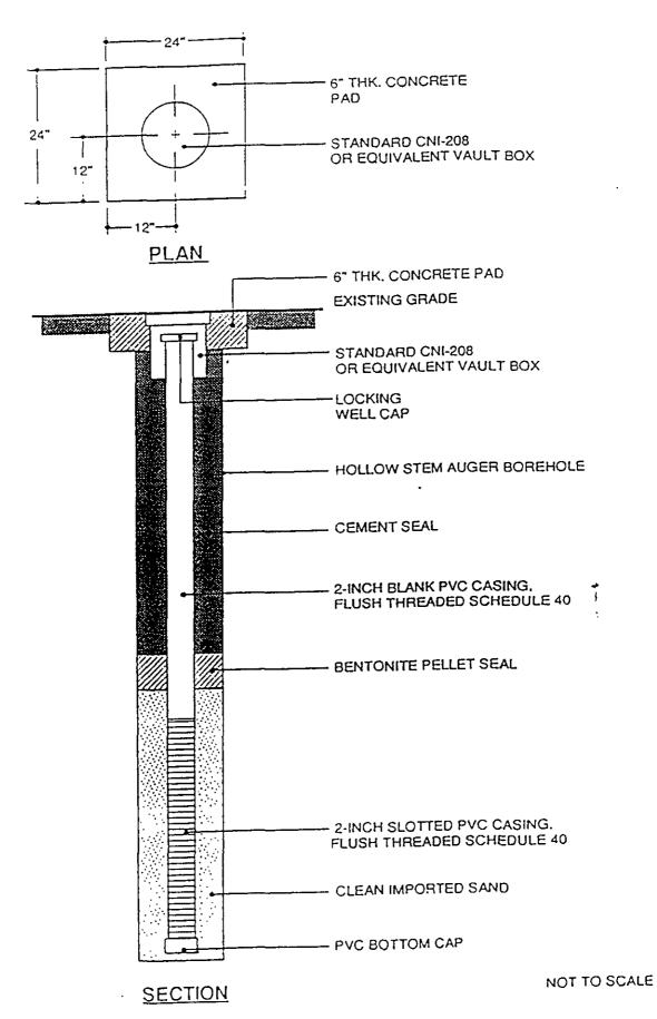
Figure A-1. Typical Monitoring Well Construction
