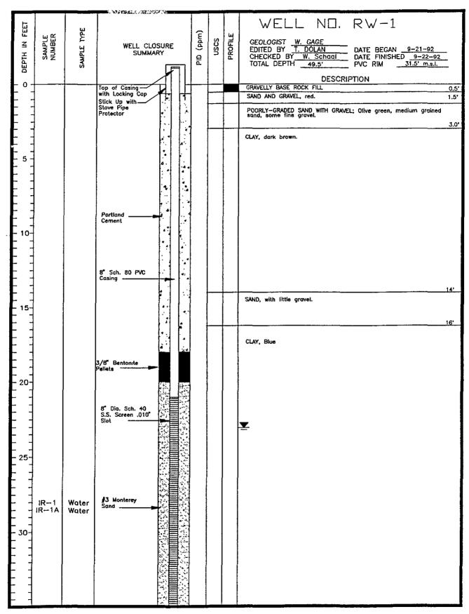
DRILLING CO.: WEST HAZMAT DRILLING DRILL METHOD: AIR ROTARY CASING HAMMER
