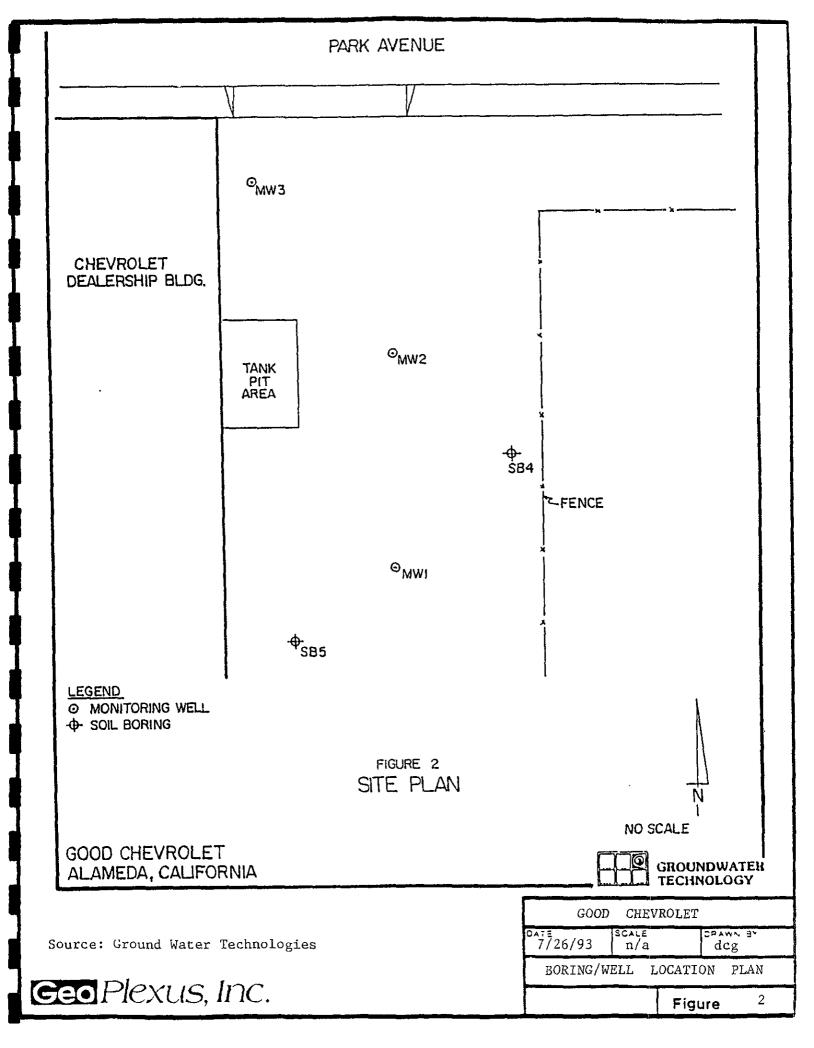
PARK STREET SIDEWALK MW-3 GOOD CHEVROLET SHOW ROOM OBSERVED VARIATION IN GROUND WATER FLOW DIRECTION APPROXIMATE SERVICE LOCATION OF AREA FORMER STORAGE TANKS GOOD CHEVROLET 0ATE 7-20-93 SCALE 1"=10' DCG GROUND WATER FLOW DIRECTION Geo Plexus, Inc. 3 **Figure**
