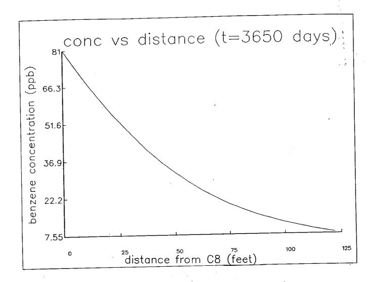
Figure 4: Plot of benzene concentration versus distance for service station 9-0504. The plot shows the concentration of benzene along a line between wells C8 and C10 at a time of ten years. The benzene source is located at well C8 and is approximated by a strip source 50 feet in length with a constant concentration of 81 parts per billion.
