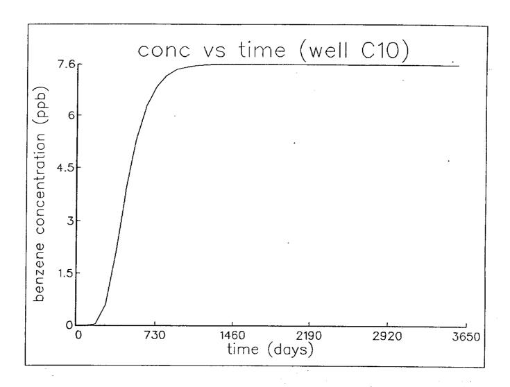
Figure 2: Plot of benzene concentration versus time for service station 9-0504. The plot shows the concentration of benzene in well C10 over a ten year period. The maximum benzene concentration that occurs in the well is approximately 8 parts per billion. The upgradient benzene source is located at well C8 and is approximated by a strip source 50 feet in length with a constant concentration of 81 parts per billion.
