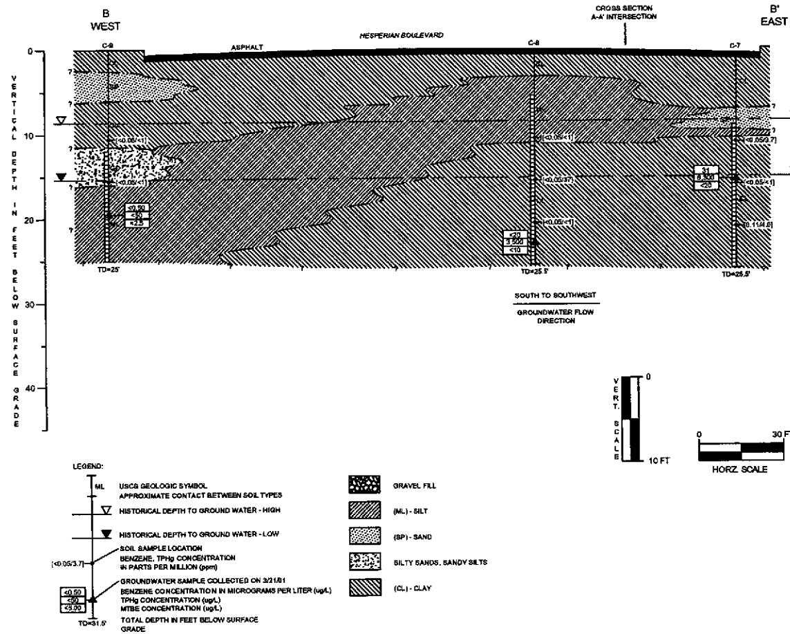
Geologic Cross Section A-A'
