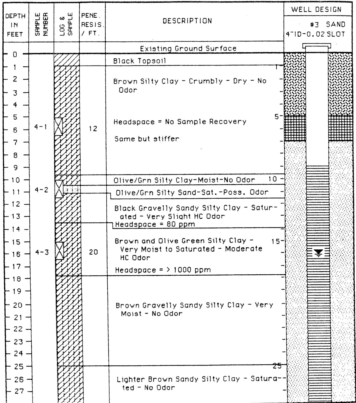
Figure 3A - Test Boring Log No. 1
