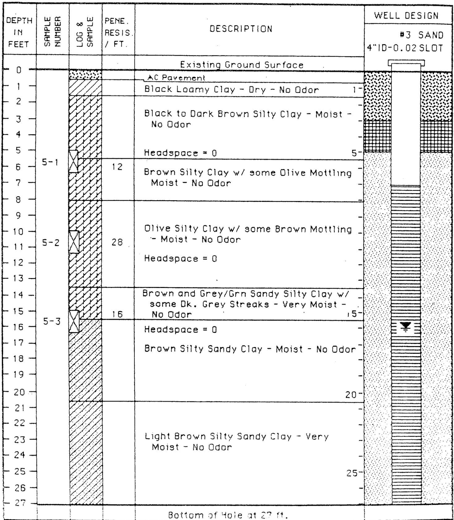
Figure 4 - Test Boring Log No. 2
