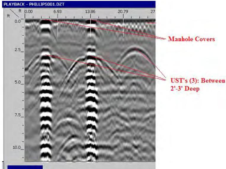
The image to the left shows example GPR data from a DIFFERENT site, where possible tank anomalies were seen in the GPR data while scanning.
