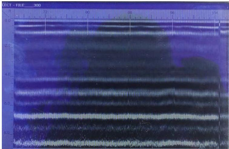
The image to the left shows “real time” GPR data while scanning on site. No apparent anomalies were seen in the GPR data to signify any possible UST’s or other related objects.
