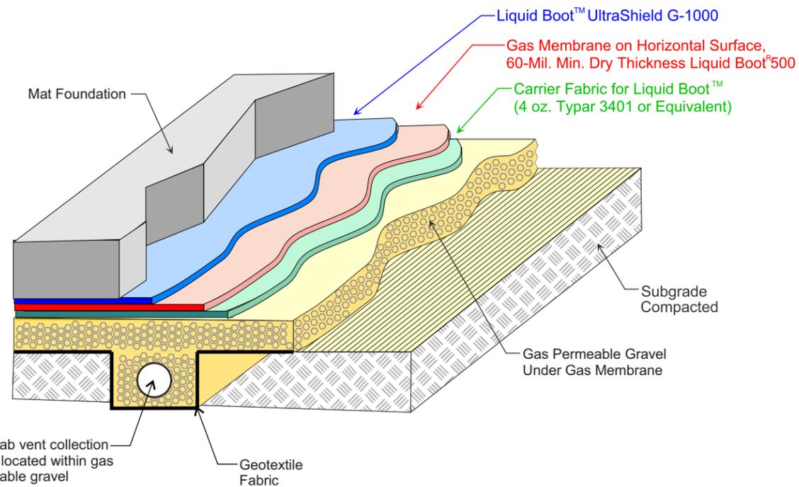
**1 Typical Vapor Barrier - Isometric View**
