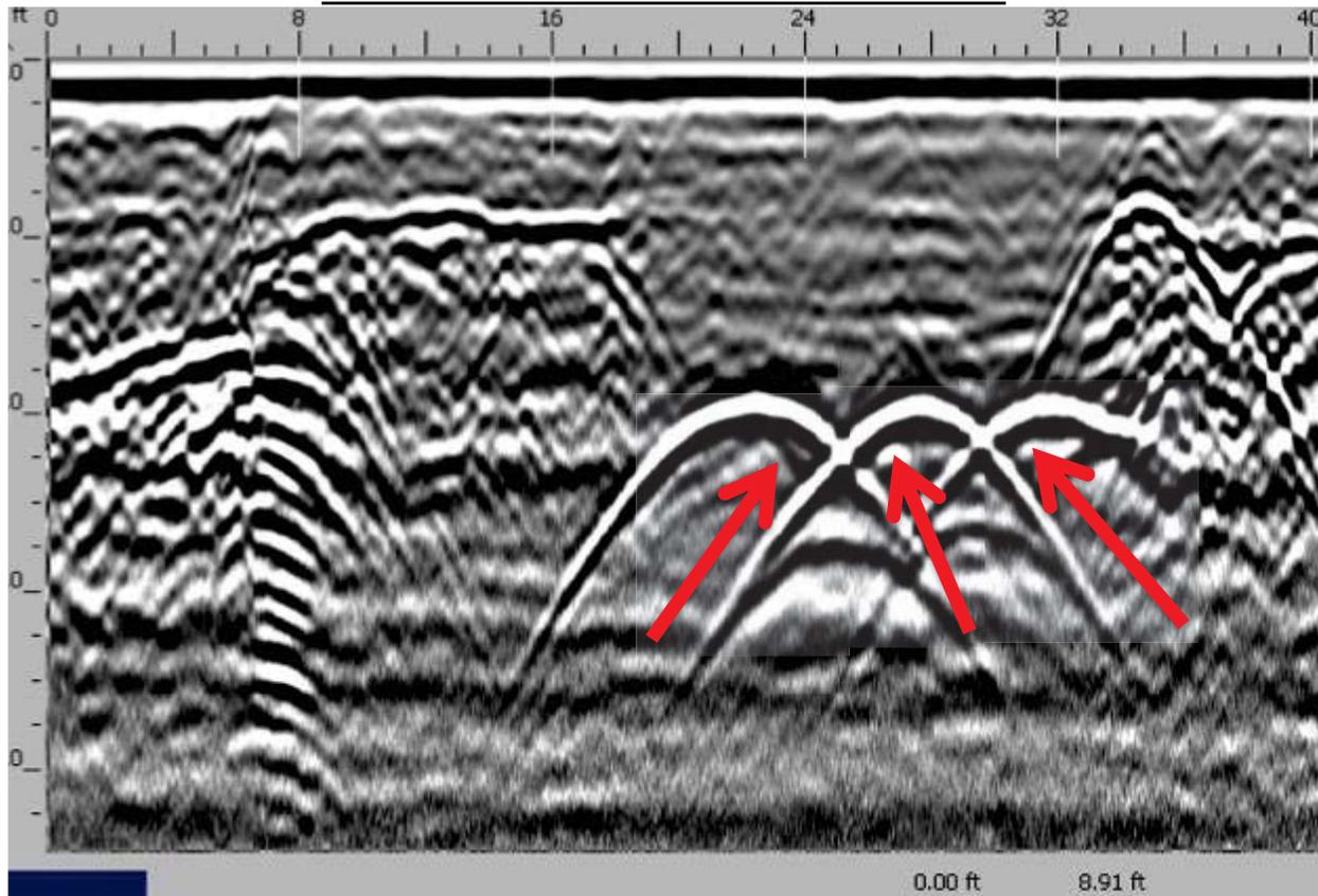
The above GPR data screen shot shows a scan across 3 tanks. The red arrows are pointing out these reactions. This scan was taken from a different site and is shown here as an example of how UST's might appear had they been found.
