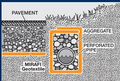
**Cut-off/Inceptor Drain Along a Roadway Or
