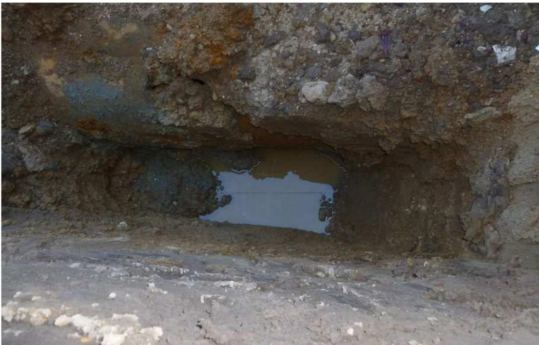
**Photo # 4. Groundwater collecting in soil sampling location at a depth of about 8 feet below the ground surface.**
