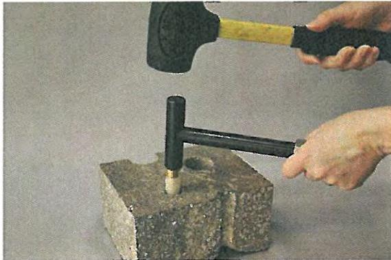
**Figure 2.** Installing the Vapor Pin™.
