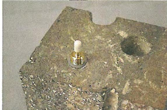
**Figure 4.** Installed Vapor Pin™.
