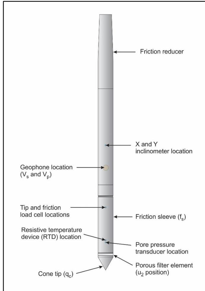
Figure CPTu. Piezocone Penetrometer (15 cm<sup>2</sup>)
