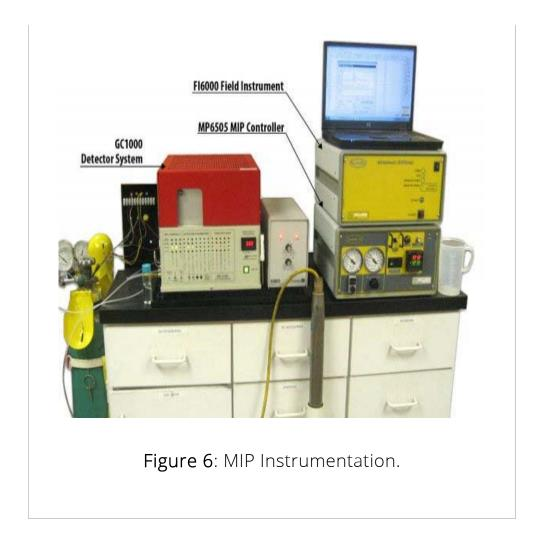
A basic set of MIP instruments is shown in **Figure 6**. These instruments include the following as labeled in the Figure:
