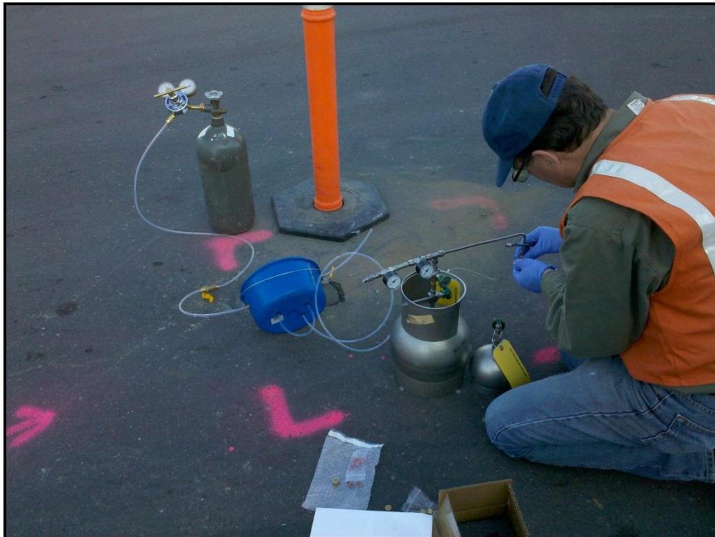
**PHOTO 7:** Setting up for soil gas sampling at SV-13. Large Summa canister is purge can; small Summa is sample can.
