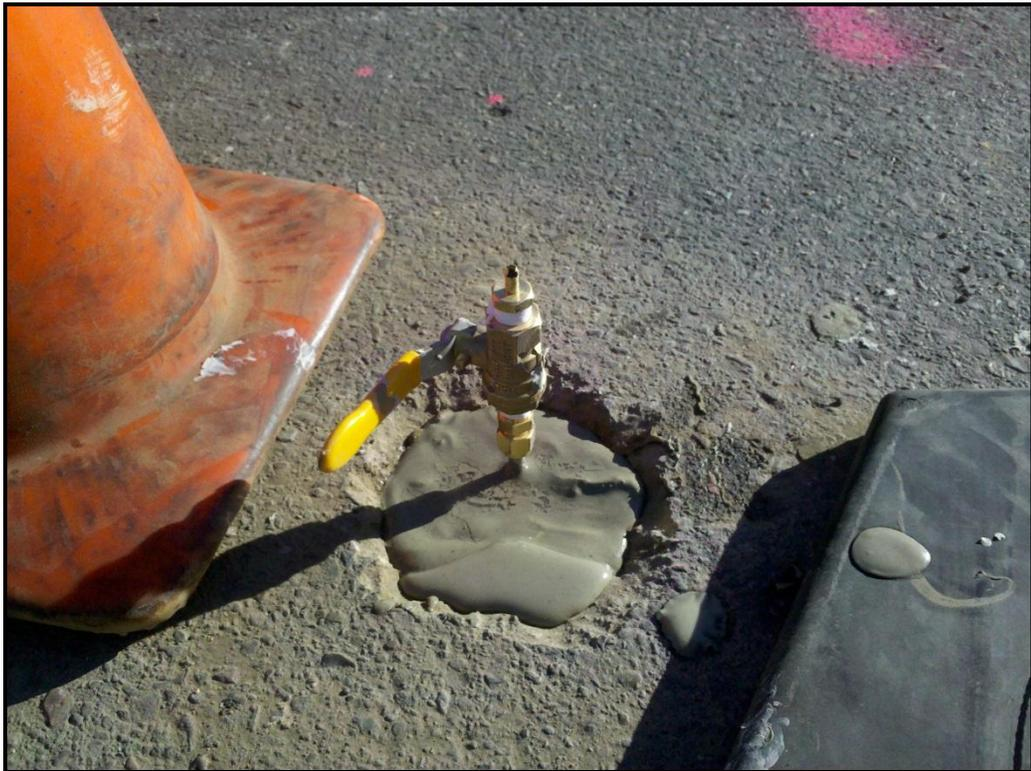
**PHOTO 4:** Typical soil gas probe surface completion.
