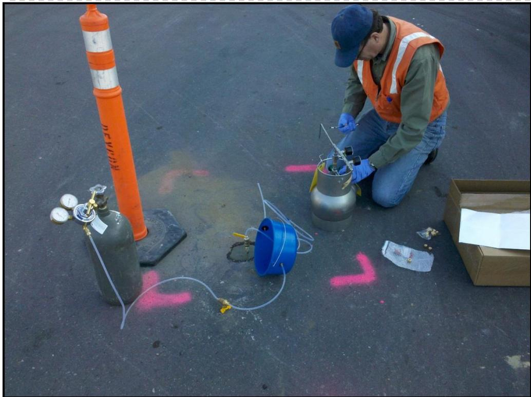
**PHOTO 6:** Setting up for soil gas sampling at SV-13. Blue bucket is helium shroud. Helium is in cylinder to the left equipped with regulator.
