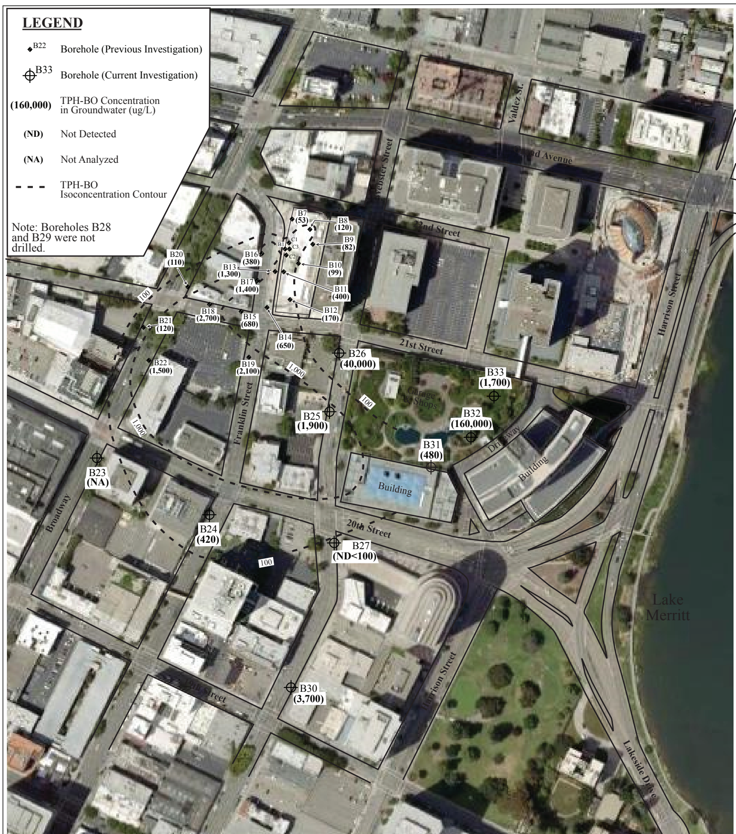
Figure 5 Site Vicinity Aerial Photograph Showing TPH-Bunker Oil in Shallow Groundwater 2100 Franklin Street Oakland, California
