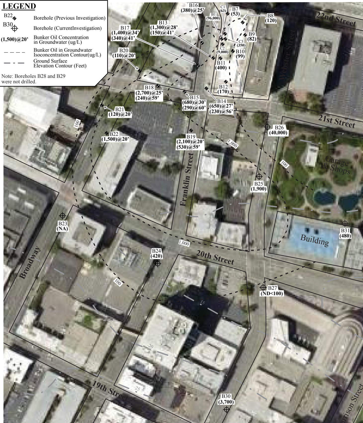
Figure 4 Site Vicinity Aerial Photograph Showing TPH-Bunker Oil in Shallow Groundwater 2100 Franklin Street Oakland, California
