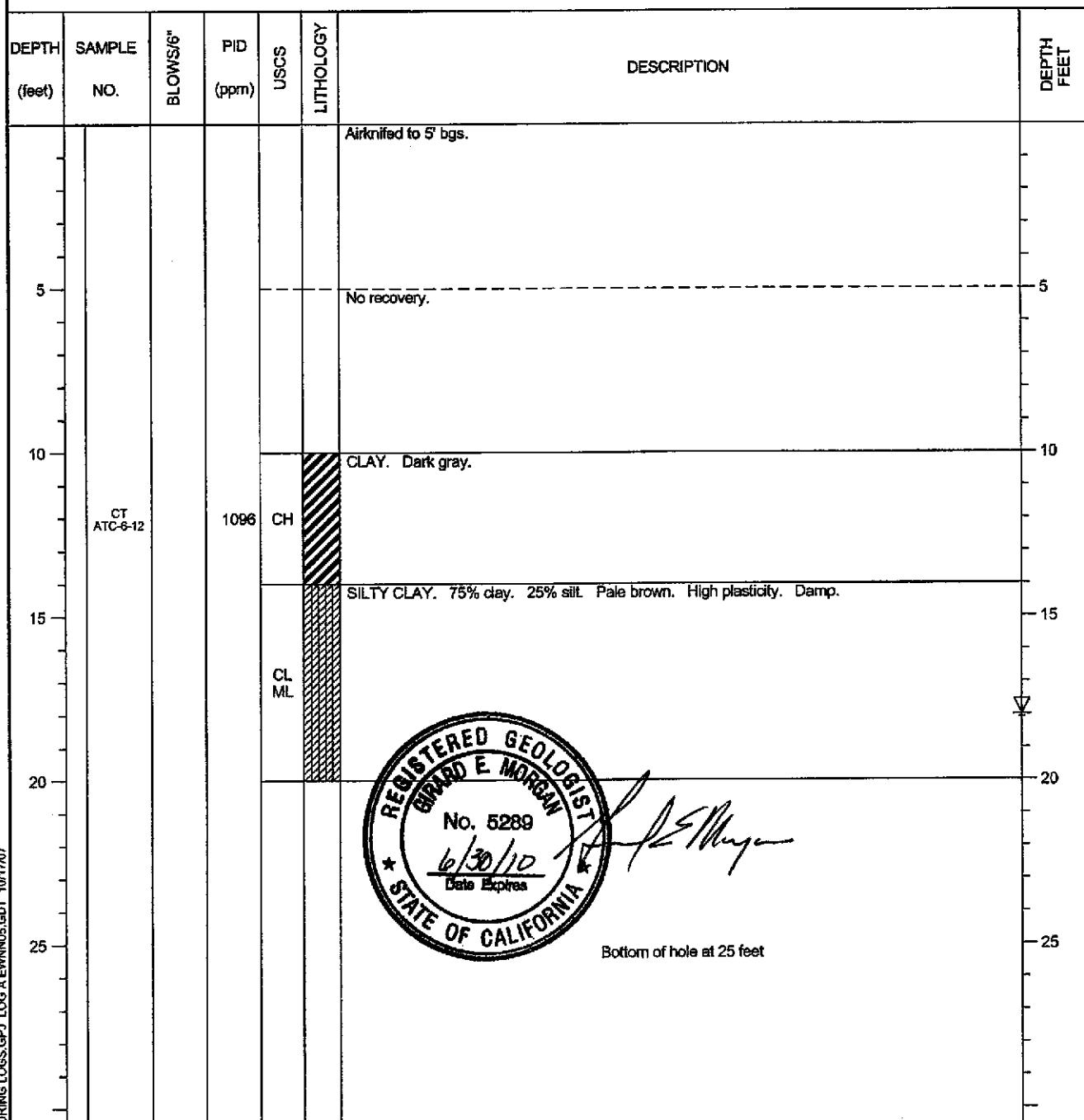
LOG A EWNNS 256277 BORING LOGS.GPJ LOG A EWNNS.GDT 10/17/07
