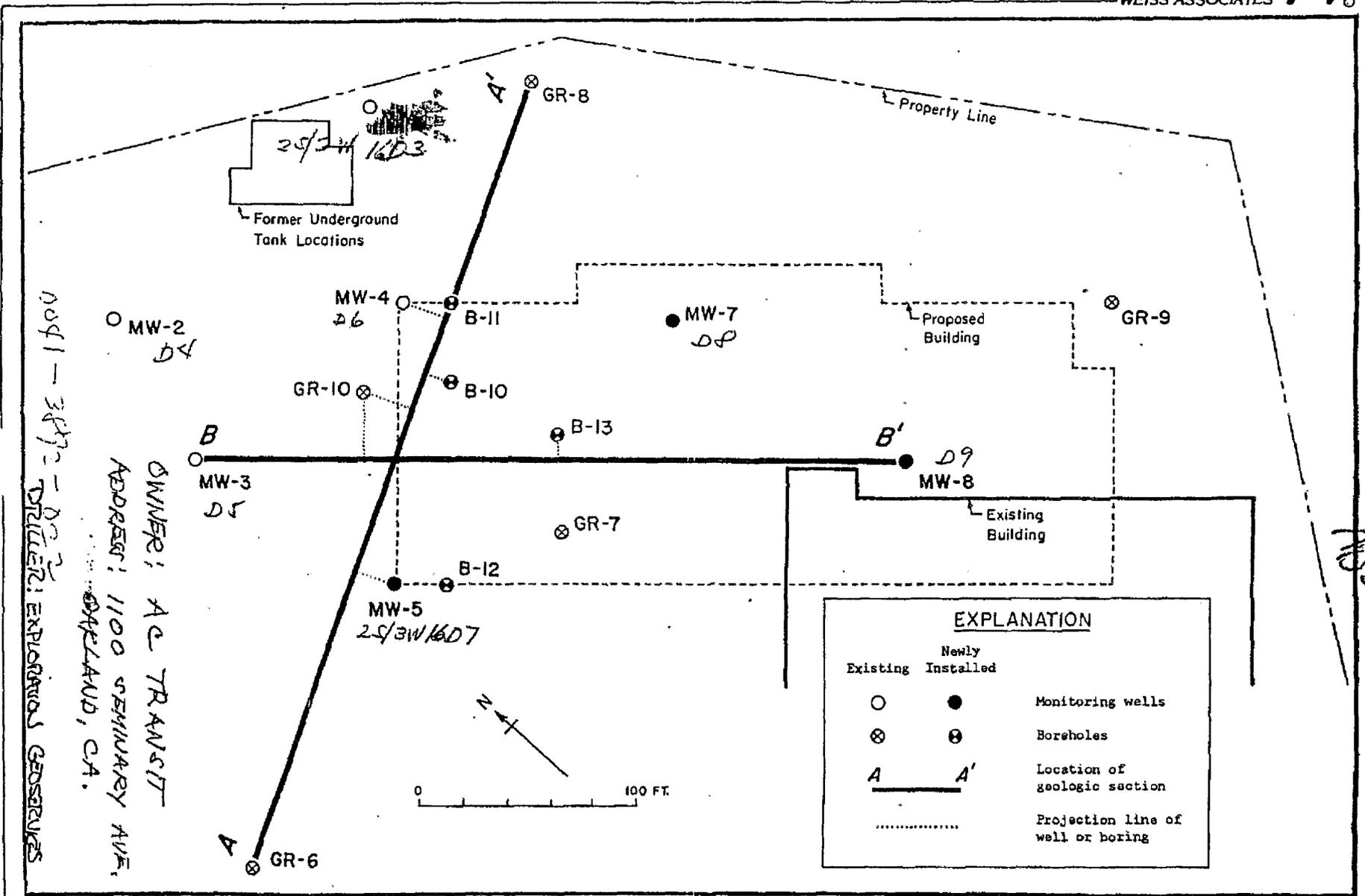
Figure 1. Location of Boreholes, Monitoring Wells, and Geologic Section - AC Transit Facility, Oakland, CA.
