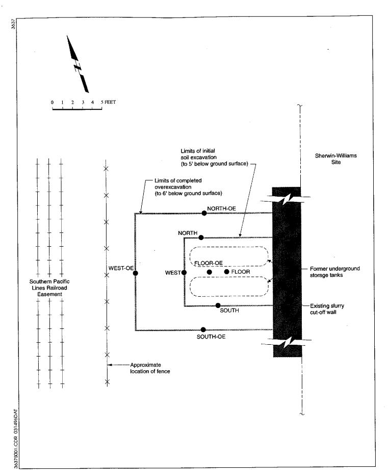
Figure 2: EXCAVATION OF USTS AND SOIL SAMPLING LOCATIONS
