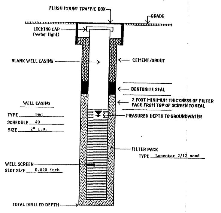
TYPICAL MONITORING WELL CONSTRUCTION DETAILS
